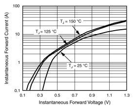
Figure 4. Typical Instantaneous Forward Characteristics
