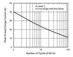
Figure 3. Maximum Non-Repetitive Peak Forward Surge Current
