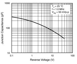
Figure 6. Typical Junction Capacitance
