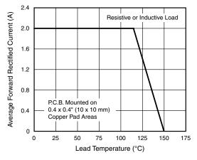
Figure 1. Forward Current Derating Curve
