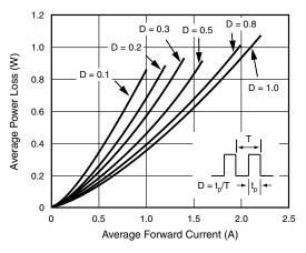
Figure 2. Forward Power Loss Characteristics
